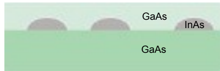
Cross-Sectional Schematic of SAQDs using GaAs substrate
