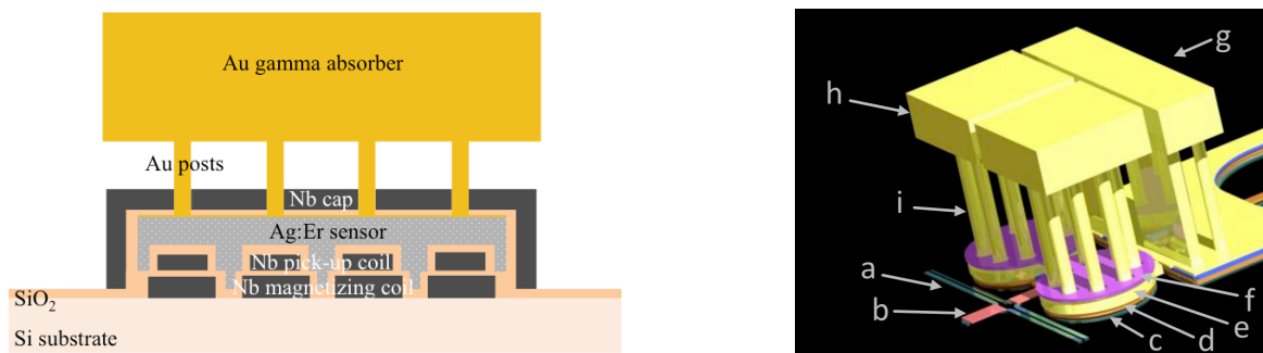
Figure 1 (left): Schematic cross-section of an MMC gamma detector (not to scale). The thick electroplated \gamma absorber is supported on top of the paramagnetic Ag:Er sensor by Au posts. The lower Nb coil is used to magnetize the sensor, and the upper coil is used to pick up the signal and couple it to the SQUID preamplifier. Figure 2 (right): A 3D schematic of an MMC shows the magnetizing circuit (a), the heat switch (b) to trap the current in the magnetizing coil (c), the sensing coil (d) below the paramagnetic Ag:Er sensor (e), the superconducting Nb cap (f) to confine the magnetizing field to the sensor (e), and the Au absorber (h) supported on Au posts (i, with height greatly exaggerated for clarity) on top of the sensor. The thermal bus (g) is designed to efficiently cool the MMC back to the base temperature of the cryostat [Boyd 2018].
