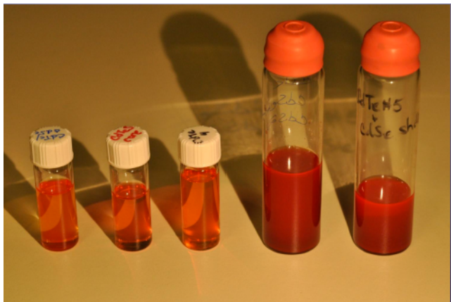
Red phosphors produced by the core-shell nanoparticle method
