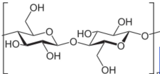
Two glucose molecules covalently linked (left). A single chain of cellulose is composed of hundreds of such glucose linkages, and individual extended cellulose molecules are hydrogen bonded (blue lines) together in plant cell walls (below).
