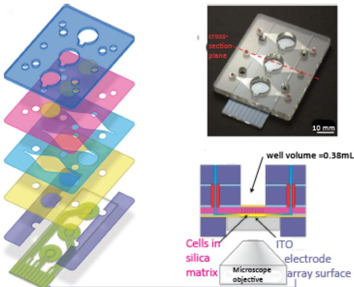
incorporated into a microfabricated device to provide the ability for three parallel methods of cell signaling upon detection of a target analyte.
