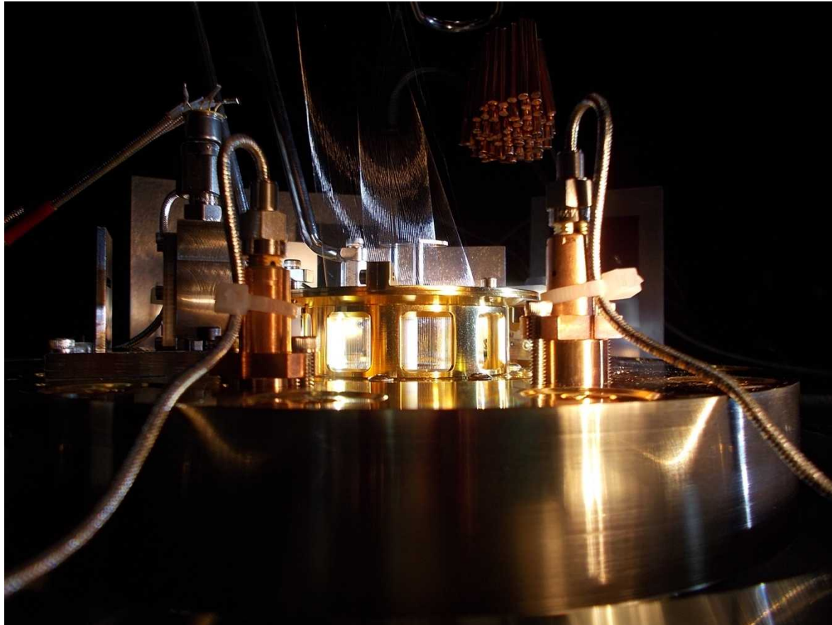
The Z-pinch radiation source used to heat the gas cell
