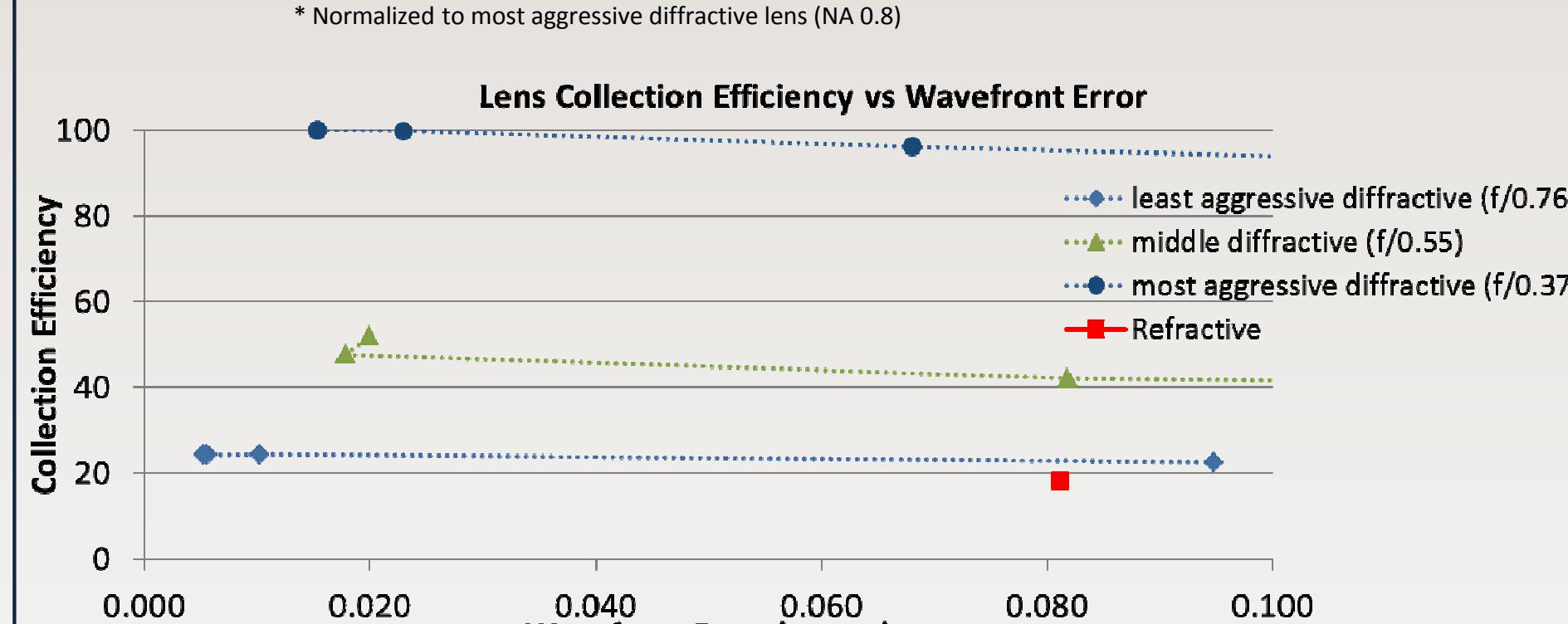
All 3 DOE options have less wavefront error and greater collection efficiency than the refractive comparison
