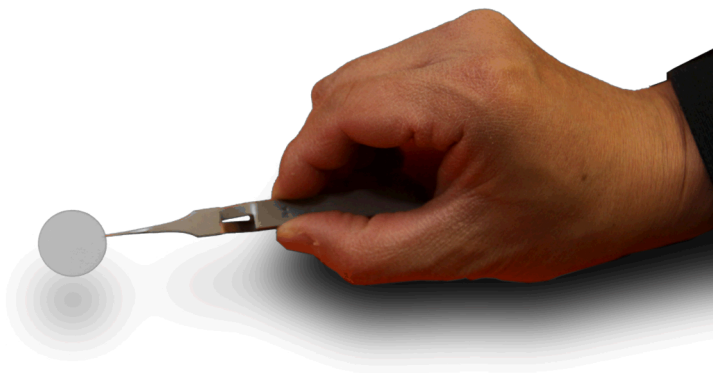
Figure 1. Nanoporous biomimetic membrane on a nanostructured support used for water desalination testing.
