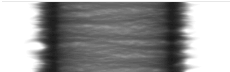
6 keV Transmission Radiographs taken of imploding liners
