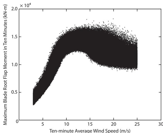
This scatter plot shows the maximum bending load on a wind turbine blade for each of more than five million simulations, plotted against the average wind speed over the duration of each simulation. This information allows designers to understand the most important wind conditions driving the design of different wind-turbine components.
