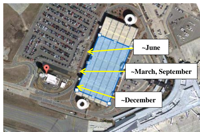
Figure 10. Approximate predicted locations and movement of glare on PV array at various times of the year.
