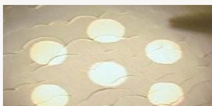
LED device made from templated films
