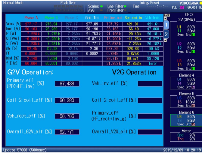
Fig. 9. Experimental results for G2V operation with state-by-stage power flow and efficiencies.
