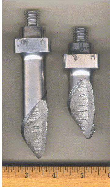
Fig. 3. Fractured contour of 7475-T7351 aluminum SNTT specimen indicates that the crack propagation orientation is perpendicular and toward the cylinder central axis.
