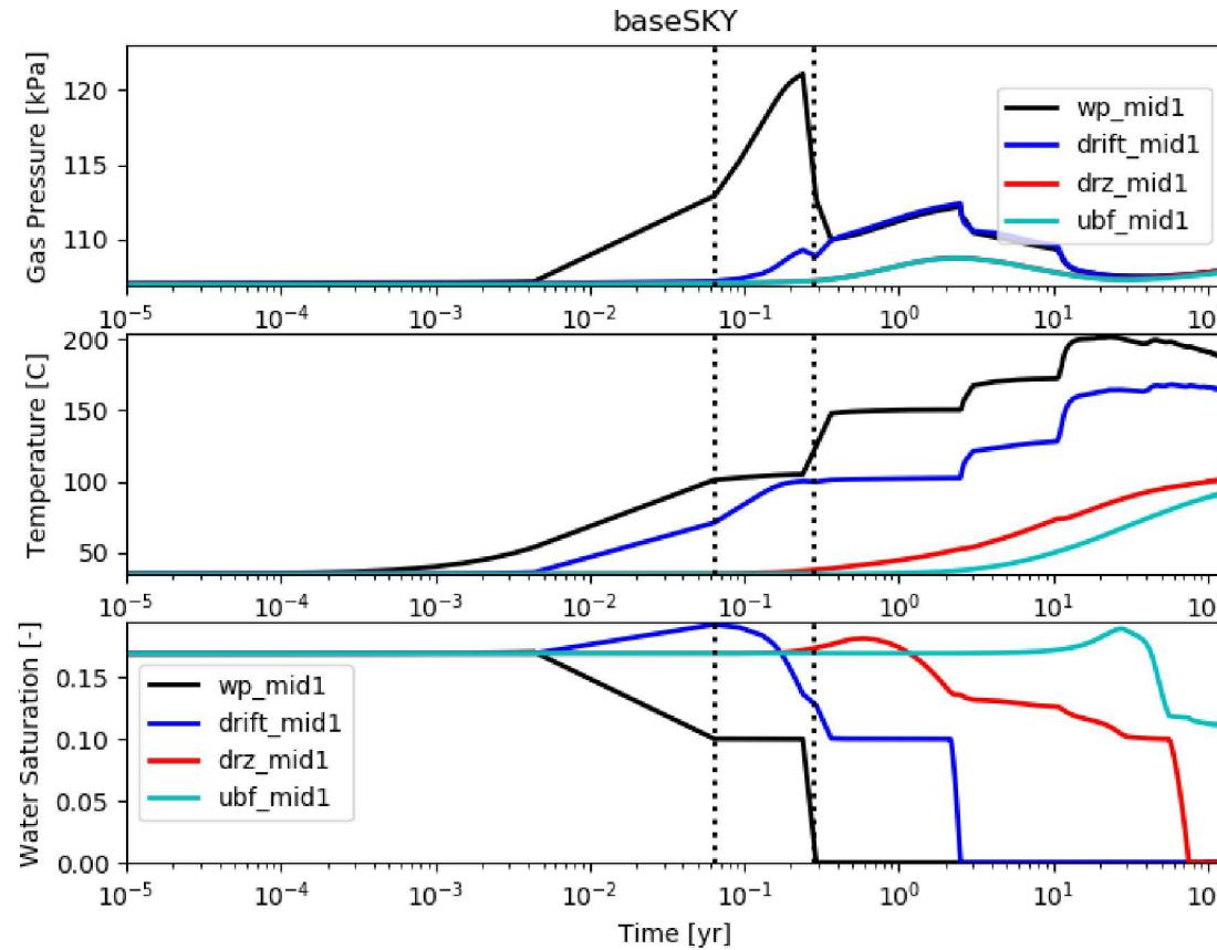
Pressure (top), Temperature (middle) and Water Saturation (bottom) near the centermost waste package as a function of log time. Values in the waste package are shown in black, in the drift next to the waste package is blue, just outside the drift is red, and the midpoint between the drift and the next drift east is cyan.
