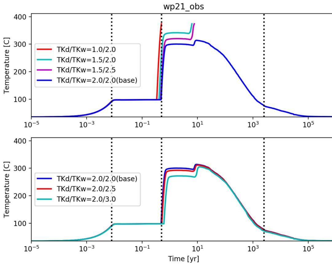
Temperature at the hottest waste package for a series of dry (top) and wet (bottom) thermal conductivities as a function of log time. Simulations stop if the critical temperature of water ( $374^{\circ}\text{C}$ ) is reached.
