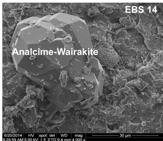
Wairakite-rich zeolite (Opalinus clay + Bentonite)
