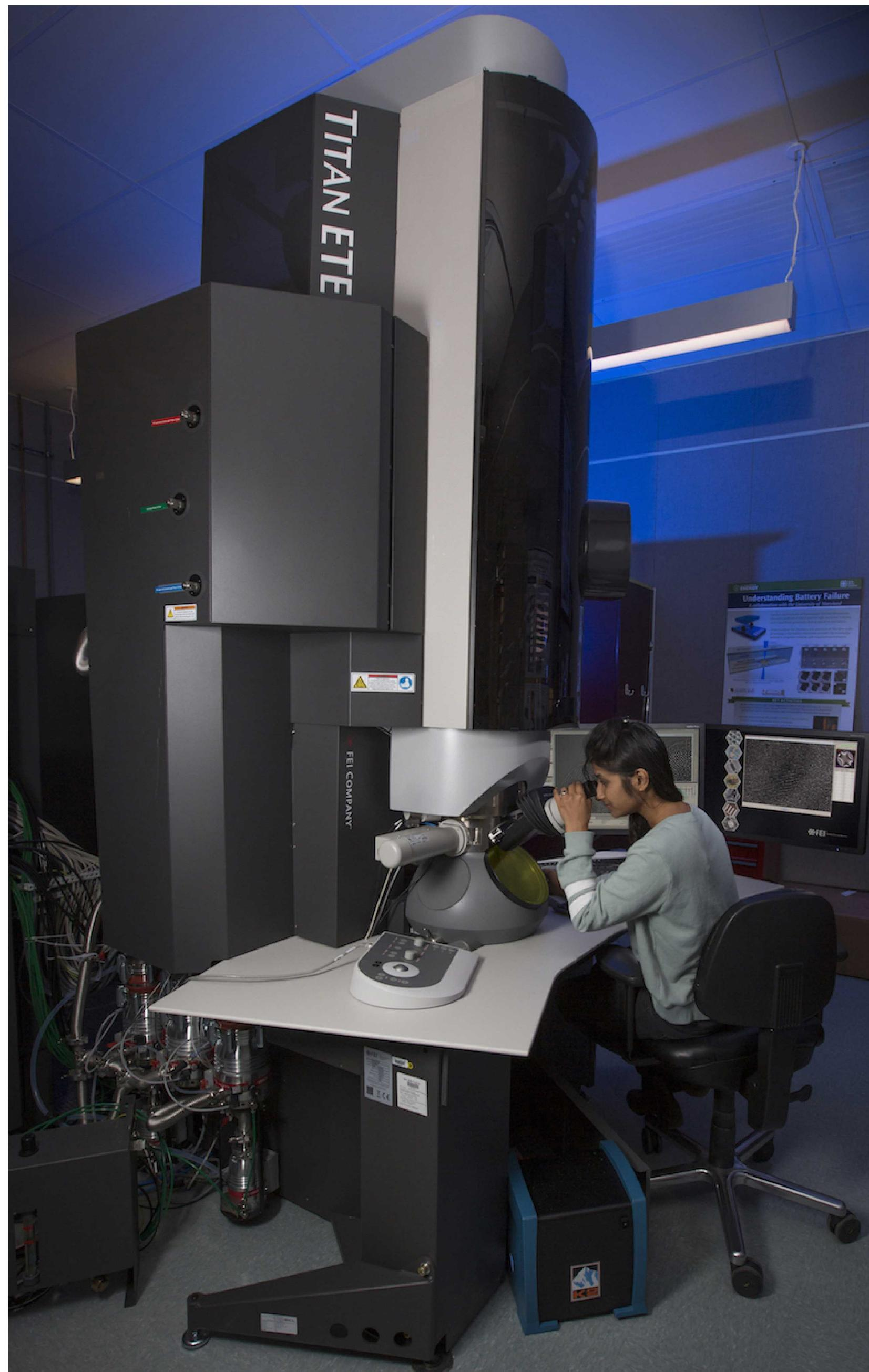
*A state-of-the-art image-corrected and monochromated Titan Environmental Transmission Electron microscope (ETEM), 300 kV, provides the capability to resolve reactions between materials and gaseous environments with atomic-resolution imaging.*
