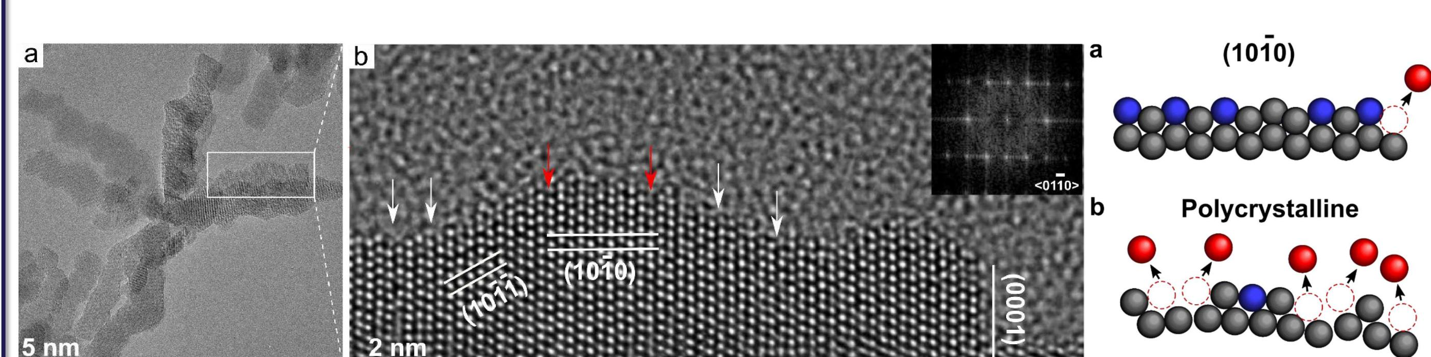
The Titan ETEM was used to characterize the surface of highly branched ruthenium (Ru) nanostructures, which display increased stability and a five-fold increase in activity for the oxygen evolution reaction (OER), when compared to polycrystalline Ru. It was shown that long, highly crystalline branches with low index crystal facets protect against Ru dissolution, a major factor reducing catalytic performance.
