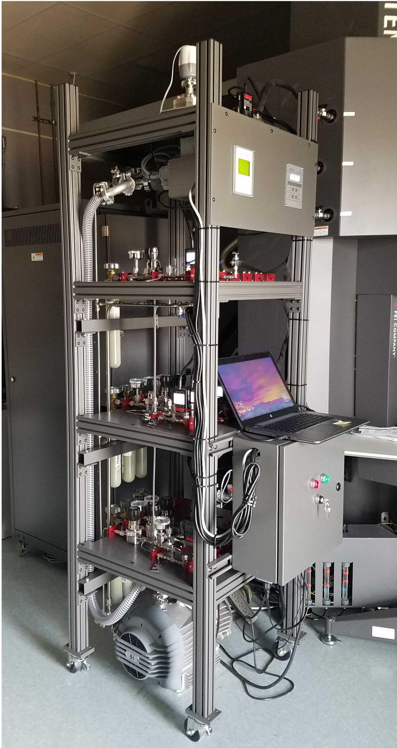
*For control over the gaseous environment in the ETEM column; including Flammable (H<sub>2</sub>, CO, methane), Inert (N<sub>2</sub>, Ar, He, CO<sub>2</sub>), and Oxidizing (O<sub>2</sub>) gases.*
