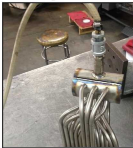
(c) The full-penetration weld was performed under a Helium atmosphere.
