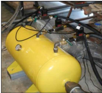
Figure 10. Alicat mass flow rate sensors attached to the three outlet manifold tank
