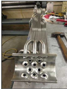
(a) 3 mm internal welds of all components
