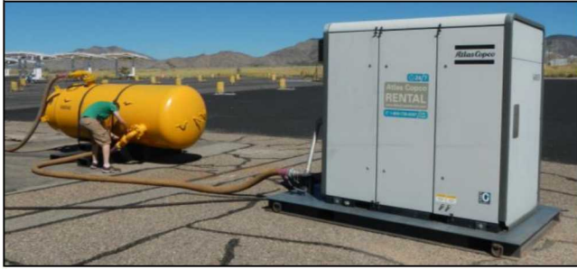
Figure 9. Air compressor (right in image) and 1000 gallon air receiver tank (yellow tank in image)
