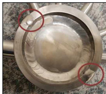
(d) The full penetration can be observed in the circled areas on the header
