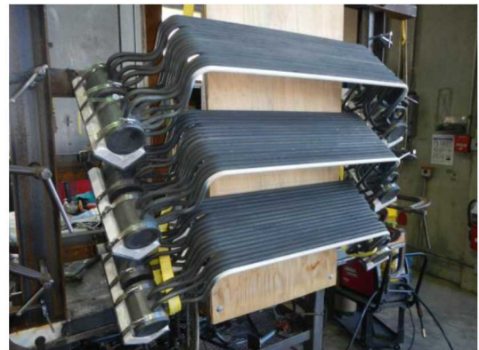
Figure 13. Bladed receiver panels with front tube painted white with VHT Flame Proof Header Paint.
