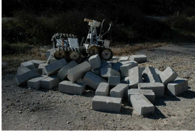
Figure 7: Gemini Scout robot operating over a block rubble pile.
