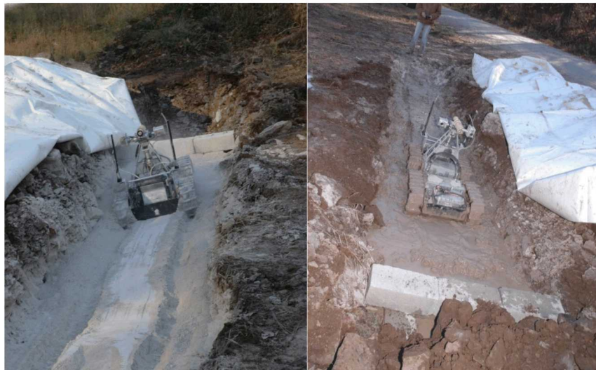
Figure 8: Gemini Scout robot driving through dry and wet rock dust.
