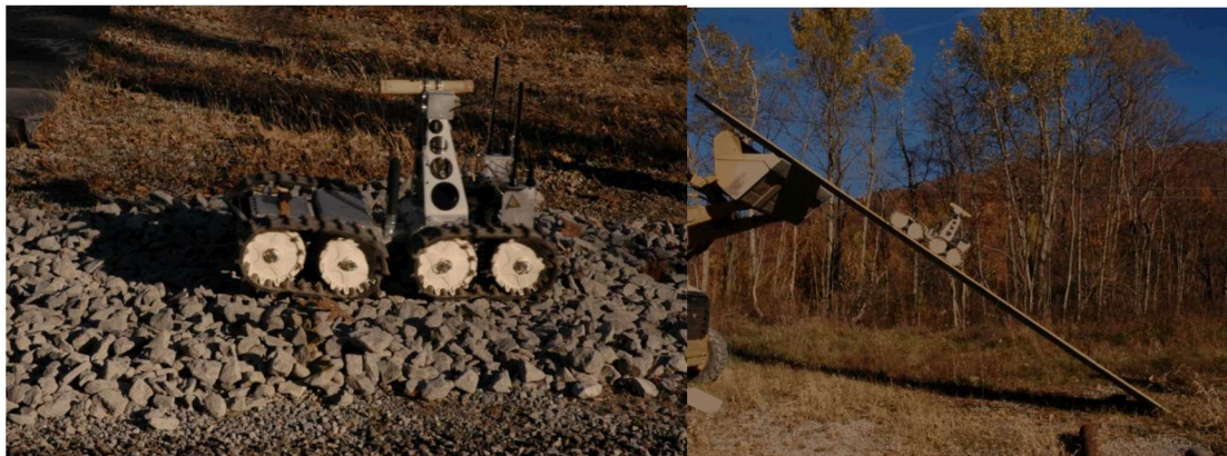
Figure 6: Gemini Scout robot operating over rough terrain and up a smooth surface.
