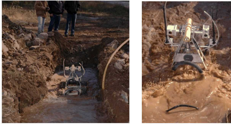
Figure 5: Gemini Scout robot operating in a water-filled dirt trench.
