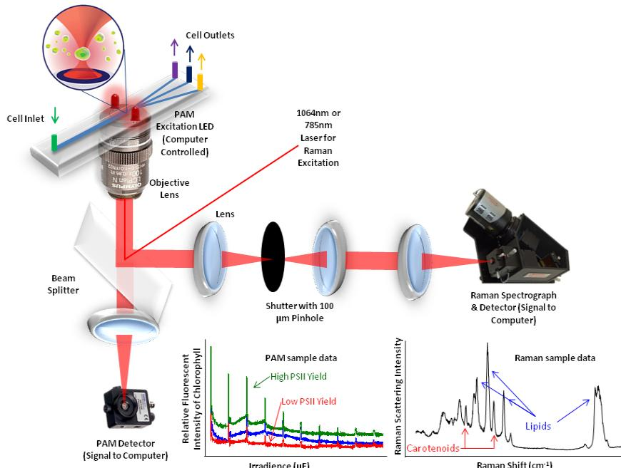
Schematic design of the multispectral microalgal optical sorter with examples of data generated (microscope, computer and connections to computer not shown). Algal cells are optically trapped (at top), above the objective lens of an inverted light microscope where they are interrogated by the laser, producing their Raman signature spectrum and by an LED, producing fluorescence that provides information on photosynthetic potency.
