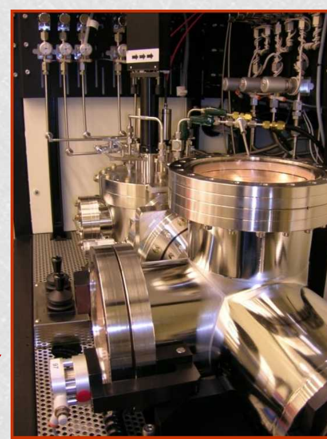
Metal-organic vapor-phase epitaxy system for growth of AlGaIn alloys and device structures
