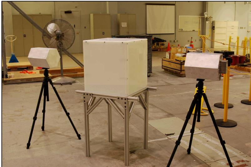
The detector is symmetric, allows for multiple sources (neutron or gamma) interrogating from opposite directions simultaneously.
