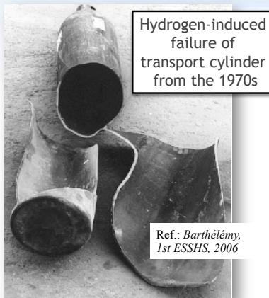
Hydrogen-induced failure of transport cylinder from the 1970s
