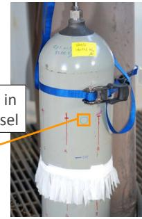
Through-wall crack in failed pressure vessel
