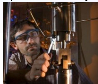
Mechanical load-frame used to characterize H 2 effects in materials
