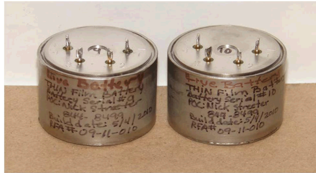
8-cell stack 1.25 inch electrode diameter
