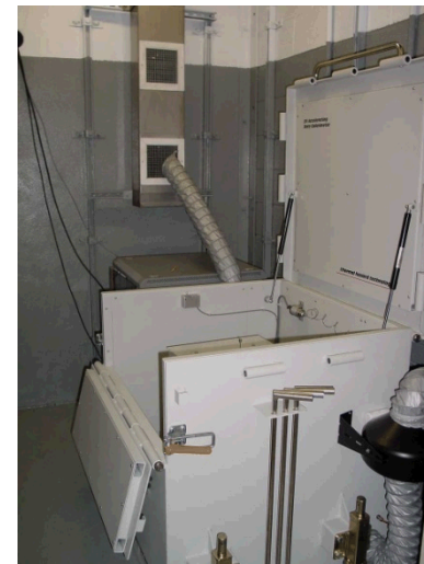
Thermal Stability (Accelerating Rate Calorimetry)
