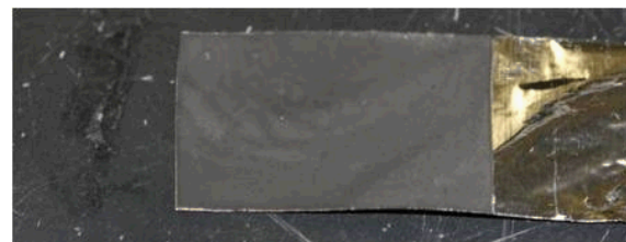
DW LiFePO 4 on current collector
