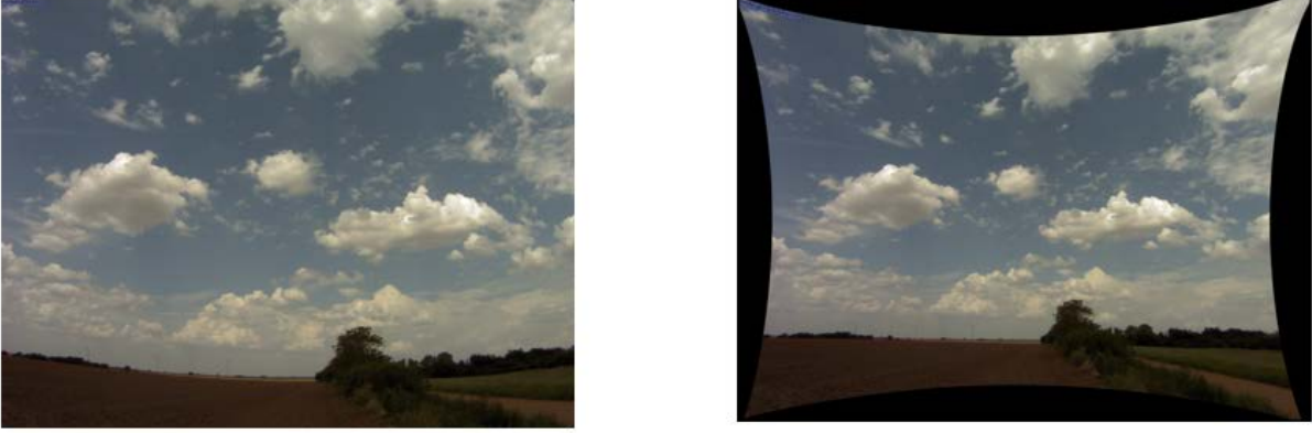
Figure 2. A sample image from the ARM stereo camera at site E45a. The image on the right is corrected for radial distortion.
