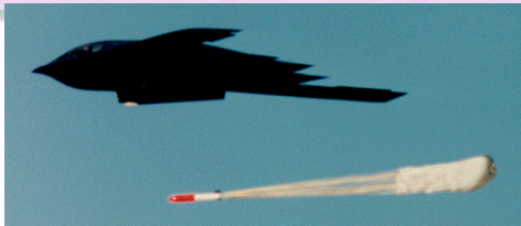
B-2 with B83 Joint Test Assembly
