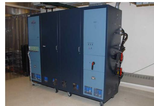
**72 V 1000 A Bitrode (2 Parallel Channels)**
