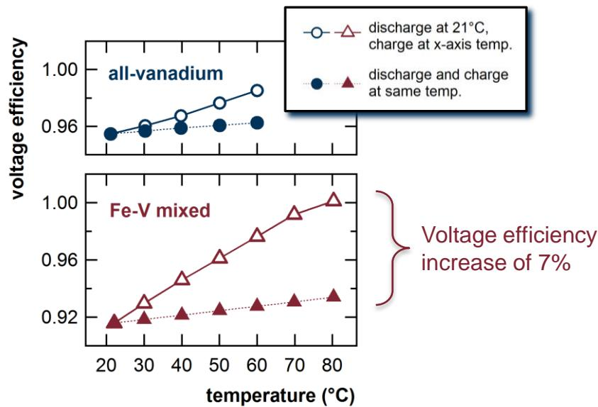
Voltage-temperature data from previous slide used to estimate the voltage efficiency at 50 mA cm<sup>-2</sup>. Major assumption is that all cell polarization is from the ohmic resistance of a Nafion 117 membrane. Nafion conductivity values from: C. H. Lee et al, *Ind. Eng. Chem. Res.* **44**: 7617 (2005)
