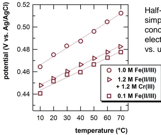
Half-cell measurements allow the simple variation of redox active concentration, supporting electrolyte concentration, mixed vs. unmixed reactants.
