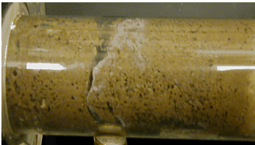
Figure 2 Soil column showing apatite crystal formed in the sediment.
