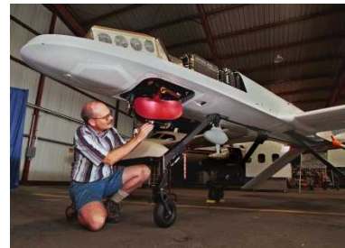
MiniSAR Mounted on Navy Tigershark UAS
