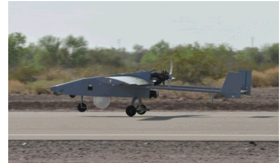
MiniSAR Mounted on Navy Tigershark UAS
