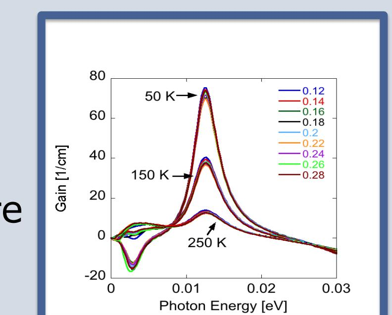
Gain spectra, showing the different gain contributions, are calculated microscopically without any fit-parameters
