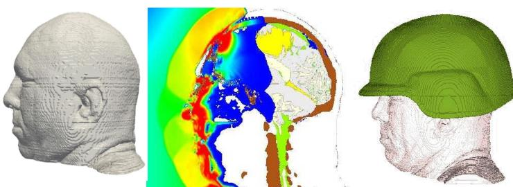
Digital head/neck model (left) exposed to frontal blast (center) & wearing Marine Lightweight Helmet (right). Computational simulation is being used to determine threshold stress values leading to Traumatic Brain Injury as part of an assessment protective helmet designs.
