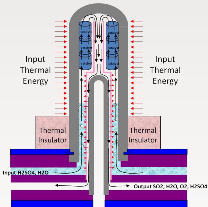
Sandia has developed a novel approach to completing the first reaction in the HyS Cycle that consists of an integrated concept for a heat exchanger/catalytic decomposer that integrates an acid boiler, superheater, and acid decomposer in a single unit. Integration of these units allows for recovery and reuse of sulfuric acid, significantly increasing the efficiency of the overall system.
