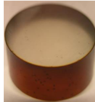
Severe degradation is limited to material surface
