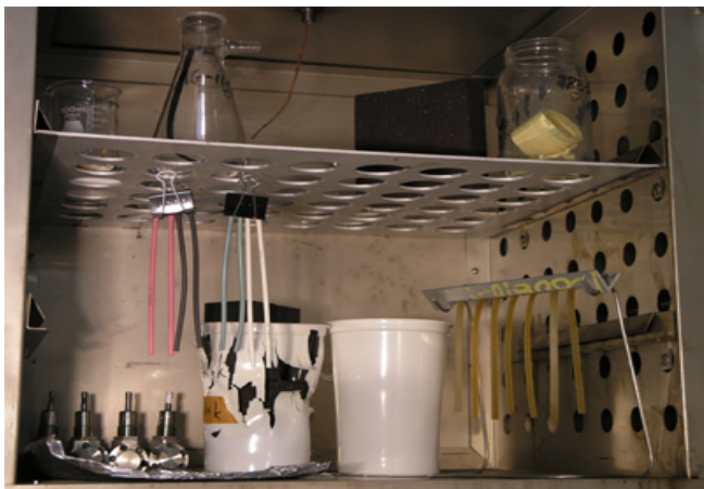
Aging ovens We select suitable temperature depending on polymers
