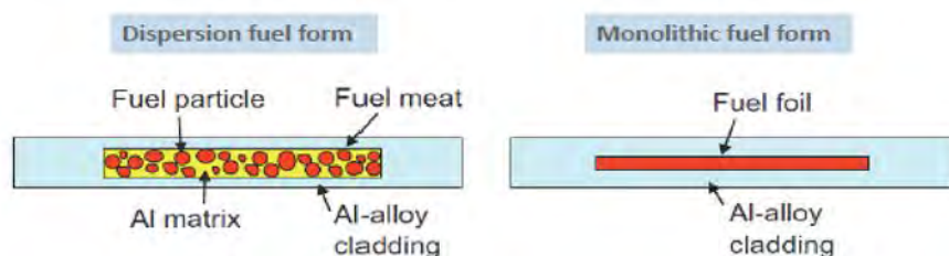
FIGURE A2.2. The Concepts of Dispersion and Monolithic Fuel Plates
