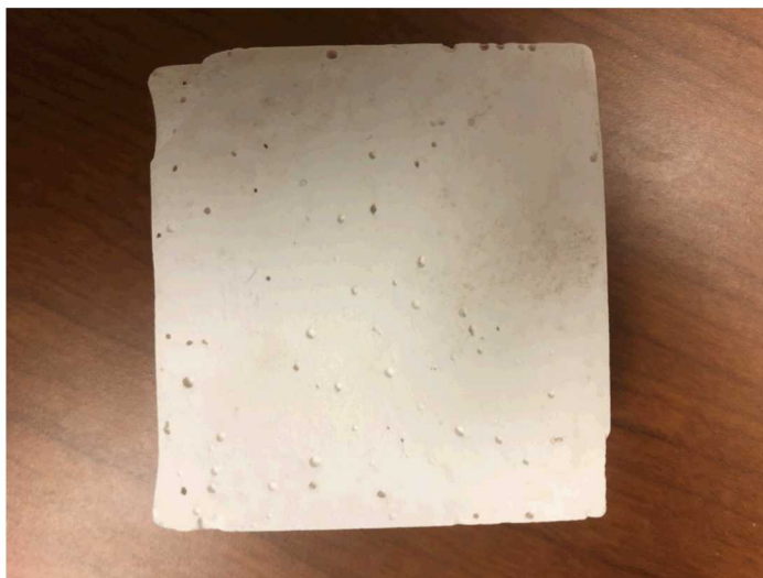
Figure 3-11. Photograph of Sample No. 1123a, a large APC monolith 4.5 cm in diameter and 4.5 cm long. Sample was sectioned in half lengthwise to reveal the presence of small isolated pores ~1mm or less in diameter.
