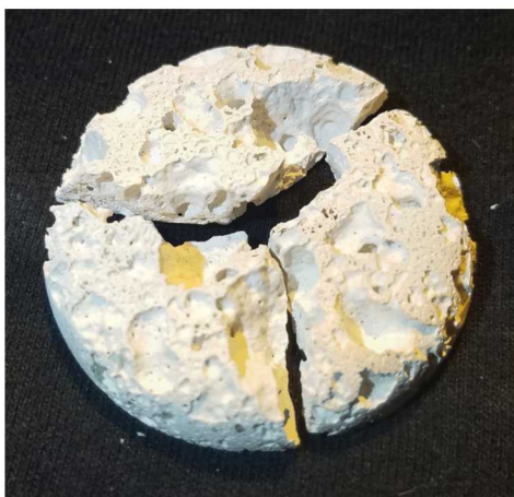
Figure 3-20. Sample 1108d is a small APC monolith 3 cm in diameter and 1 cm thick. Note numerous large and irregular pores as large as 1 cm in diameter.
