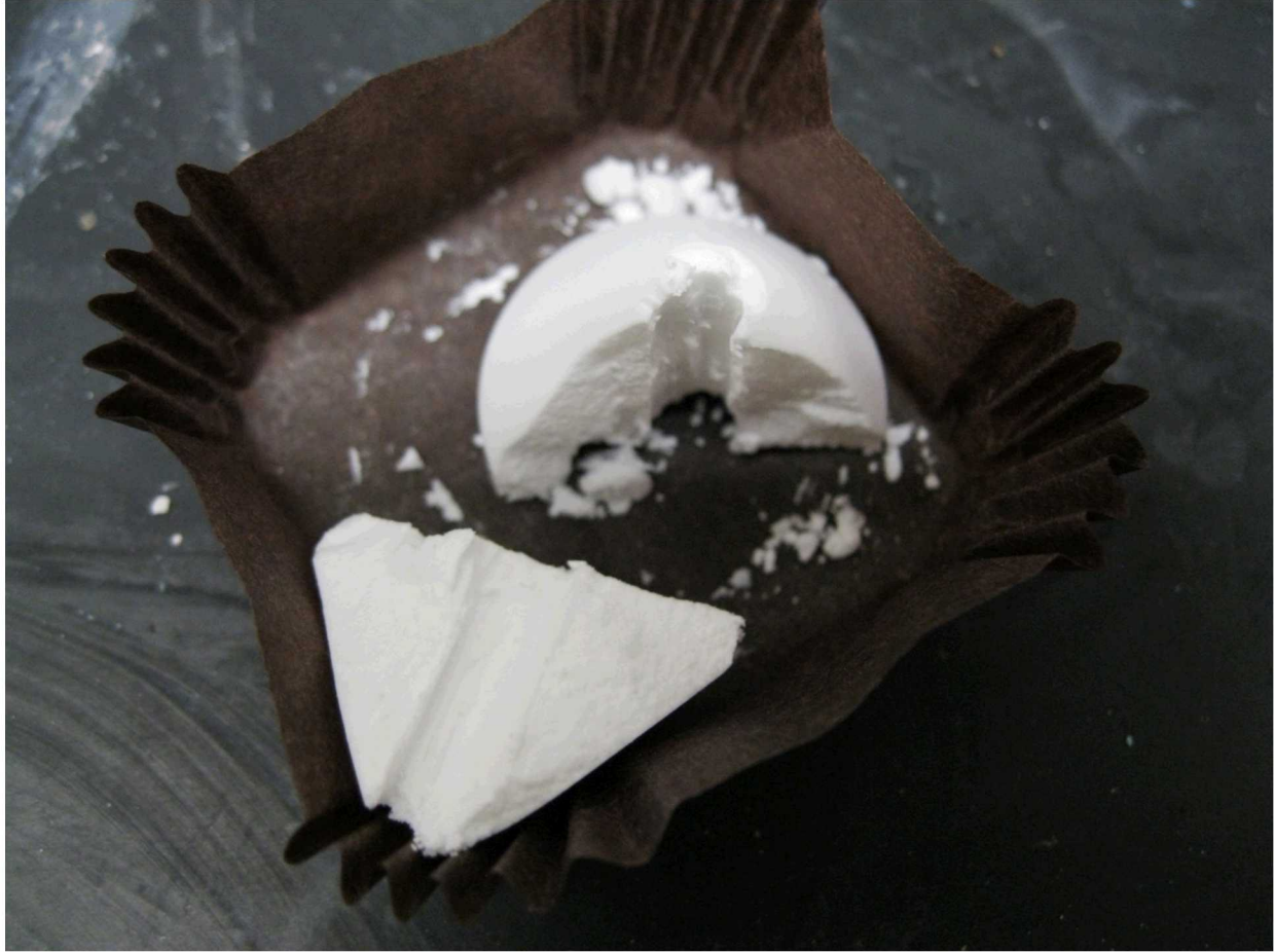
Figure 5-12. CPC sample prepared using buffered phosphate (equimolar ratios of \text{K}_3\text{PO}_4 , \text{K}_2\text{HPO}_4 , \text{KH}_2\text{PO}_4 , and \text{H}_3\text{PO}_4 ) solution. A stir rod left in the slurry was easily removed and resulted in a fracture across the entire piece, likely due to excessive salt content.
