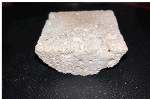
Figure 3-22. Photograph of Sample No. 1206 that is 4.5 cm in diameter and 4.5 cm long. Sample was sectioned in half lengthwise to reveal the numerous large pores up to 8 mm in diameter.
