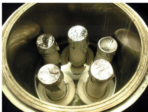
Figure 3-9. Parr reactor with glass tubes containing \text{Al}_2\text{O}_3 / \text{H}_3\text{PO}_4 / \text{H}_2\text{O} slurries.
