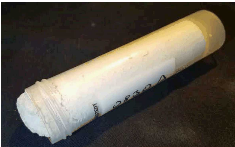
Figure 3-31. Photograph of Sample No. 0830a-50mL. Note the monolith has expanded above the top of the 50 mL centrifuge tubes.
