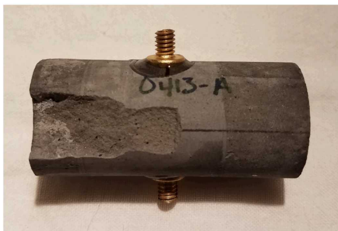
Figure 4-10. Photograph of Sample No. 0413a (after mechanical testing). Sub-millimeter pores can be observed appearing as very dark specks.
