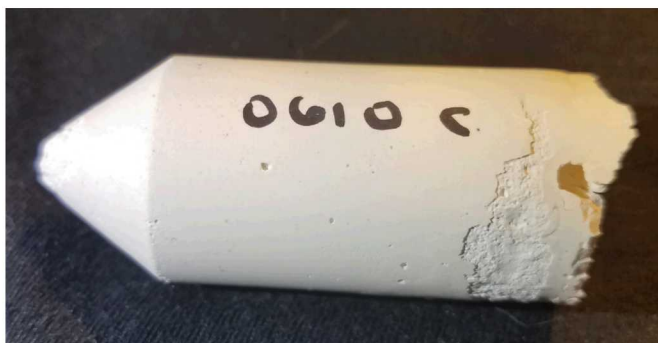
Figure 3-27. Photograph of Sample No. 0610c. Sample is 2.5 cm in diameter and ~ 6 cm long. Isolated pores that are evident are 1 mm or less in diameter.
