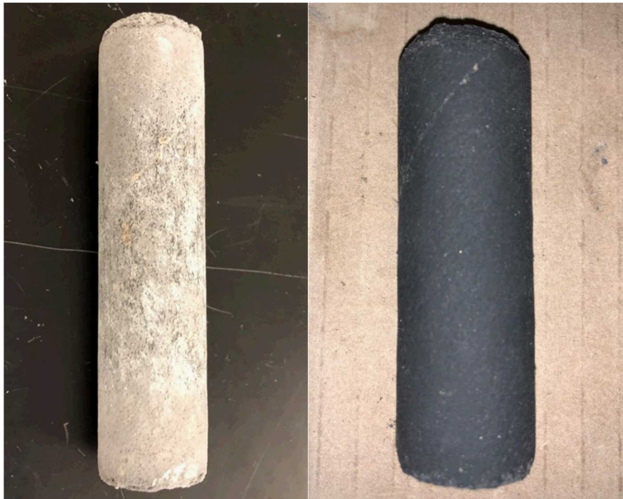
Figure 6-2. Fabricated baseline MKP cement core (left), and baseline MKP cement with boron carbide fabricated core (right). Samples are approximately 2.54 cm (1 in) in diameter and 10.16 cm (4 in) long.
