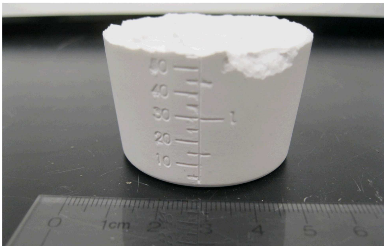
Figure 5-16. Demolded monolith showing features from mixing beaker.
