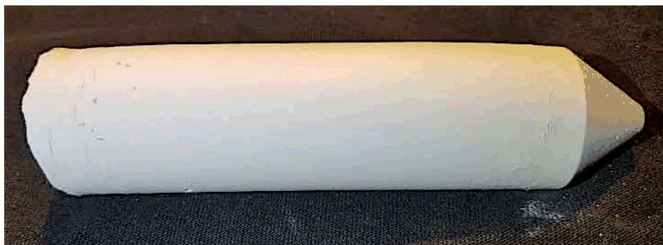
Figure 3-32. Photograph of Sample No. 0830c-50mL \text{Al}_2\text{O}_3 /Metakaolin combined with \text{H}_3\text{PO}_4/\text{NaH}_2\text{PO}_4 \cdot \text{H}_2\text{O} .
