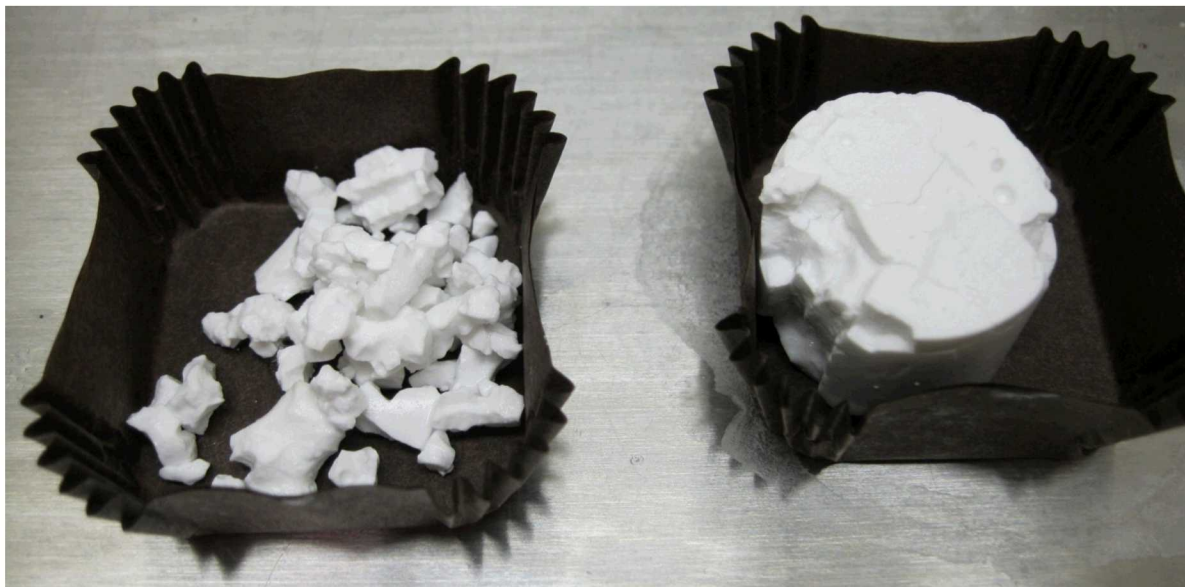
Figure 5-14. Sample monoliths after the hydrothermal stability test. Low (1M) concentration K_3PO_4 solution-derived samples survived (right), while high concentration (2 M) derived samples did not (left).
