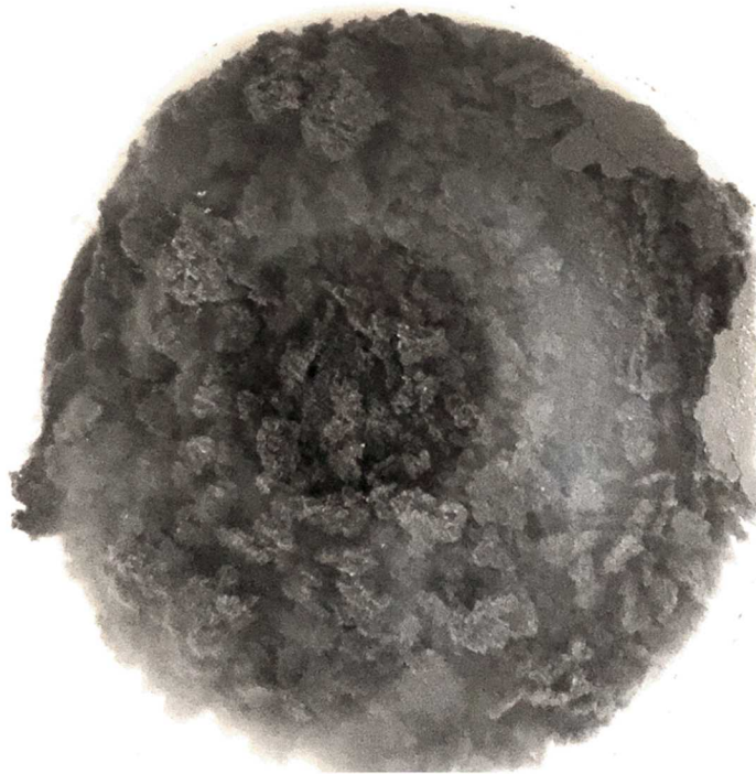
Figure 6-3. MKP cement sample with boron carbide ( H_2O added at 19% by weight of powder) after immersion in for 24 hours in distilled water.
