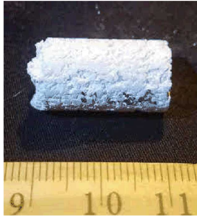
Figure 3-4. Photograph of Sample No. 1124a. The sample is 2 cm long and 1.2 cm in diameter.
