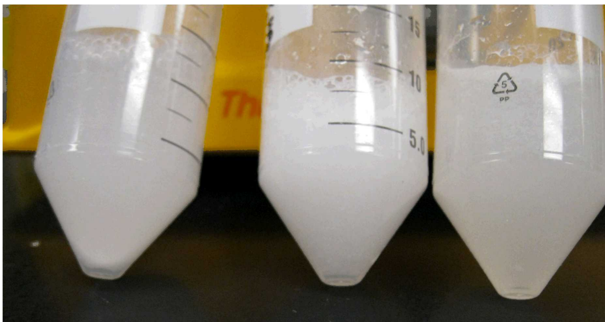
Figure 5-7. Solubility tests (left to right) of 1 mmol DDDA in 1 M K 2 HPO 4 , 2.5 M K 2 HPO 4 and 5 M K 2 HPO 4 .
