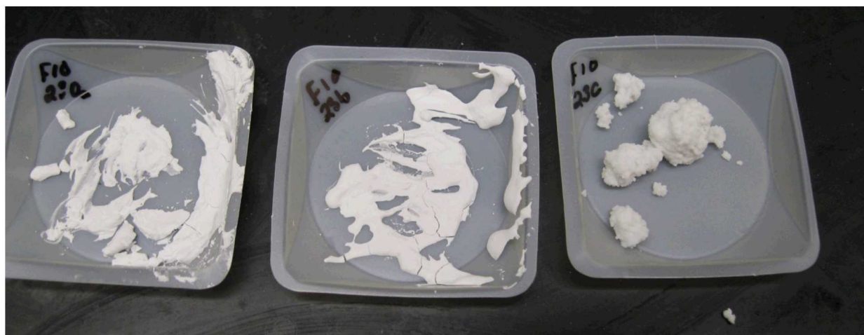
Figure 5-9. Dried aliquots of (left) tetracalcium phosphate in water, (center) tetracalcium phosphate in 1 M K_3PO_4 , and (right) tetracalcium phosphate in levulinic acid mixed with 1 M K_3PO_4 .
