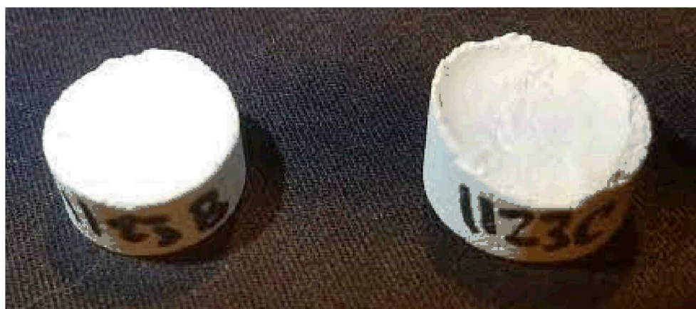
Figure 3-2. APC sintered monolith Sample Nos. 1123b and 1123c using organo-phosphonic acids. Samples are 2.5 cm in diameter and 1.3 cm tall.
