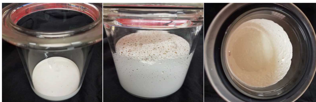
Figure 3-8. Photographs of the \text{Al}_2\text{O}_3 / \text{H}_3\text{PO}_4 / \text{H}_2\text{O} slurry before (left), during (center), and after (right) degas.
