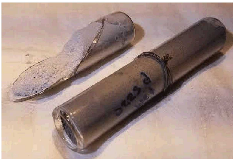
Figure 4-3. Photograph of Sample Nos. 0223b-H and 0223d-H. 0223b-H (top) is a crumbly powder that did not survive removal from the tube while 0223d-H is a wet unconsolidated powder. The sample tubes are 7.5 cm long and 2 cm OD.
