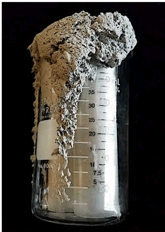
Figure 7-6. Photograph of Sample No.0823g. Note that the talc-based material foamed considerably upon preparation.
