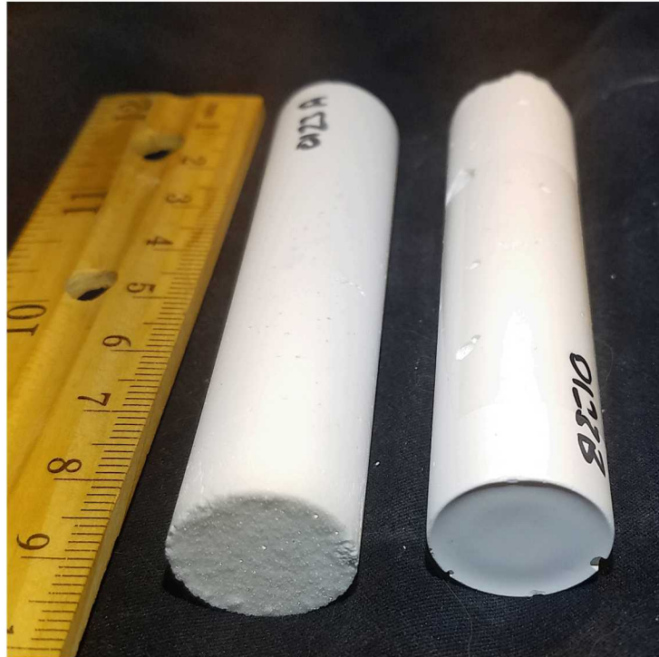
Figure 3-14. Photograph of Sample Nos. 0123a and 0123b. Note the top surface of the monolith (left) is covered with small crystals.
