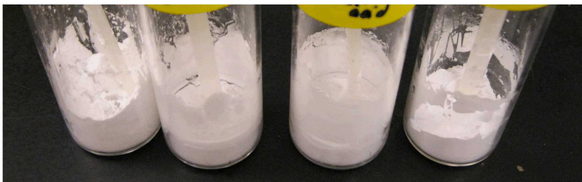
Figure 5-3. Dental cement samples prepared using bifunctional or trifunctional carboxylic acid as a moderator. From left to right, samples are 1% malonic acid, 1% citric acid, 0.5% citric acid and 0.5% malonic acid.
