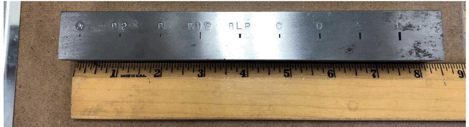
Calibration block with machined defects
