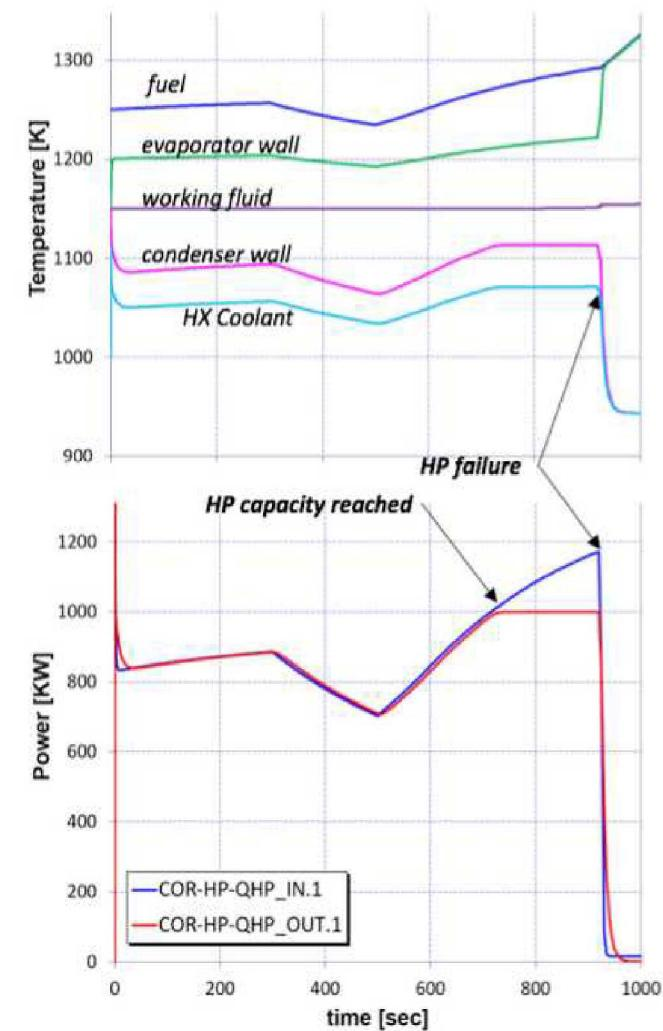
Illustrative output (temperatures and in/out power) from a slow transient of a simple HP test problem
