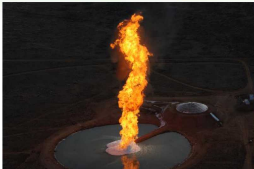
LNG fires on water at Sandia Albuquerque
