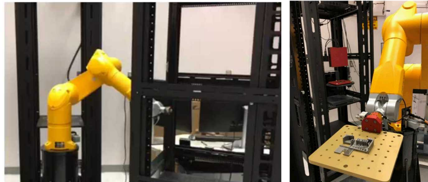
robotic work cell for material characterization
