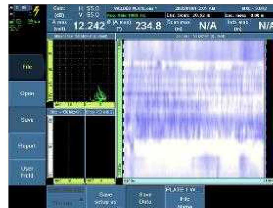
Top scan of weld: No flaw indications.
