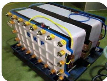
32 KW Stack Rongke Power/UET 120 mA/cm 2 Meter size stack
