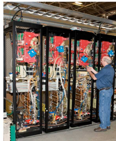
1 MVA Single-Phase Solid State Power Substation [1]
