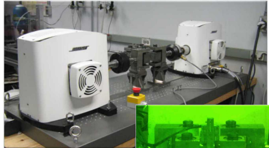
CIRFT tester out of the hot cell (above) and in the hot cell (right) testing High-Burnup Fuel samples.
