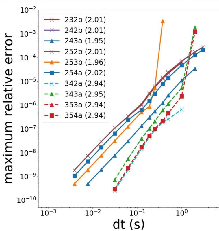
(Left) Error in solution of 5 hour run of DCMIP 2012 non-hydrostatic gravity wave test case, 1.25km horizontal resolution, 20 vertical levels. Hyperviscosity and vertical remap were disabled.
