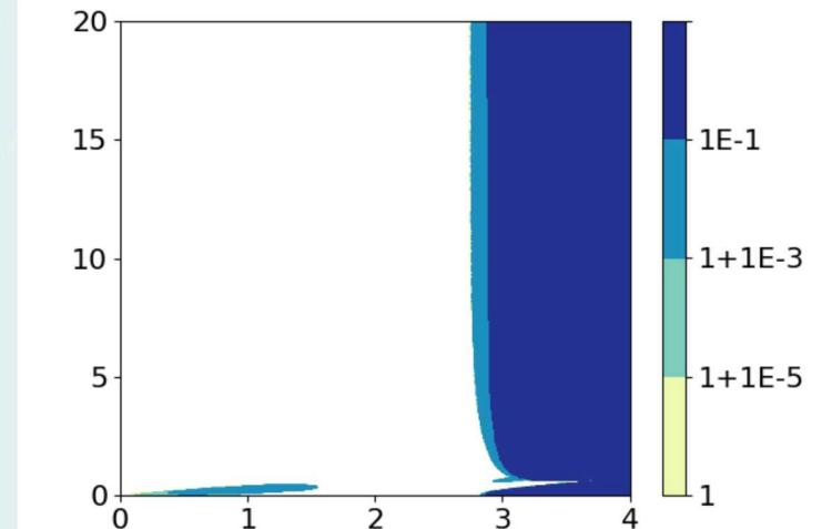
H-stability regions of the IMKG242a (left) and IMKG242b (right) methods. Max. stable time-steps at v-to-h aspect ratios 1/100, 1/10, and 1: IMKG242a 175, 17.5, 2.25; IMKG242b 225, 27.5, 2.75. Hydrostatic time-steps 275, 27.5, 2.75.
