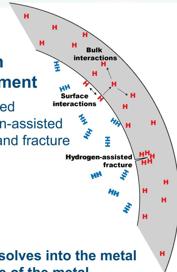
Hydrogen dissociates on metal surfaces, dissolves into the metal lattice, and changes the mechanical response of the metal
