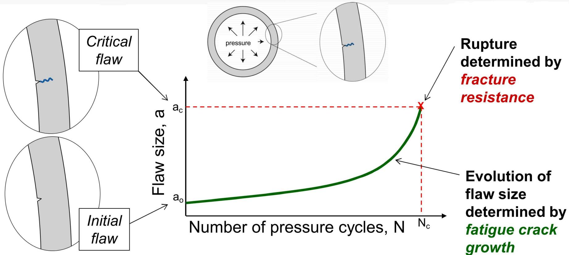
ASME B31.12 describes rules for hydrogen pipelines with reference to ASME BPVC Section VIII, Division 3, Article KD-10
