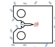
**Fracture resistance of pipeline steels in H<sub>2</sub> is greater than driving force on semi-elliptical cracks**
