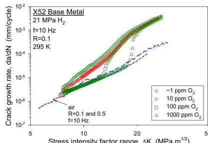
– **Oxygen can mitigate the effects of hydrogen in some cases, which perhaps can be exploited**
