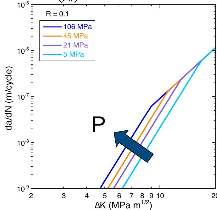
The bound at high  $\Delta K$  is dependent on  $R$  (i.e.,  $K_{max}$ ), but not sensitive to pressure
