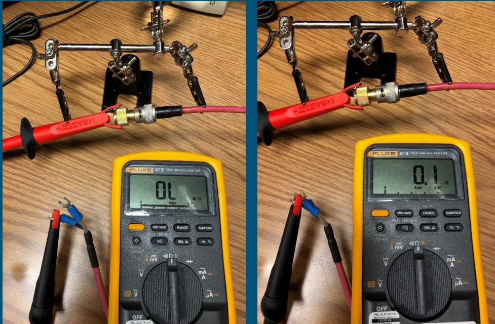
Bench demonstration of contact on center conductor before shield.
