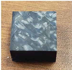
Section of the fiber reinforced composite for serial sectioning.
