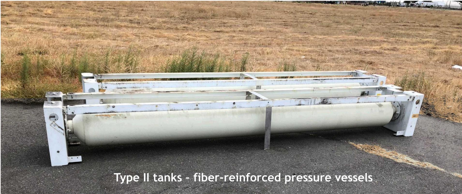
Type II tanks - fiber-reinforced pressure vessels
